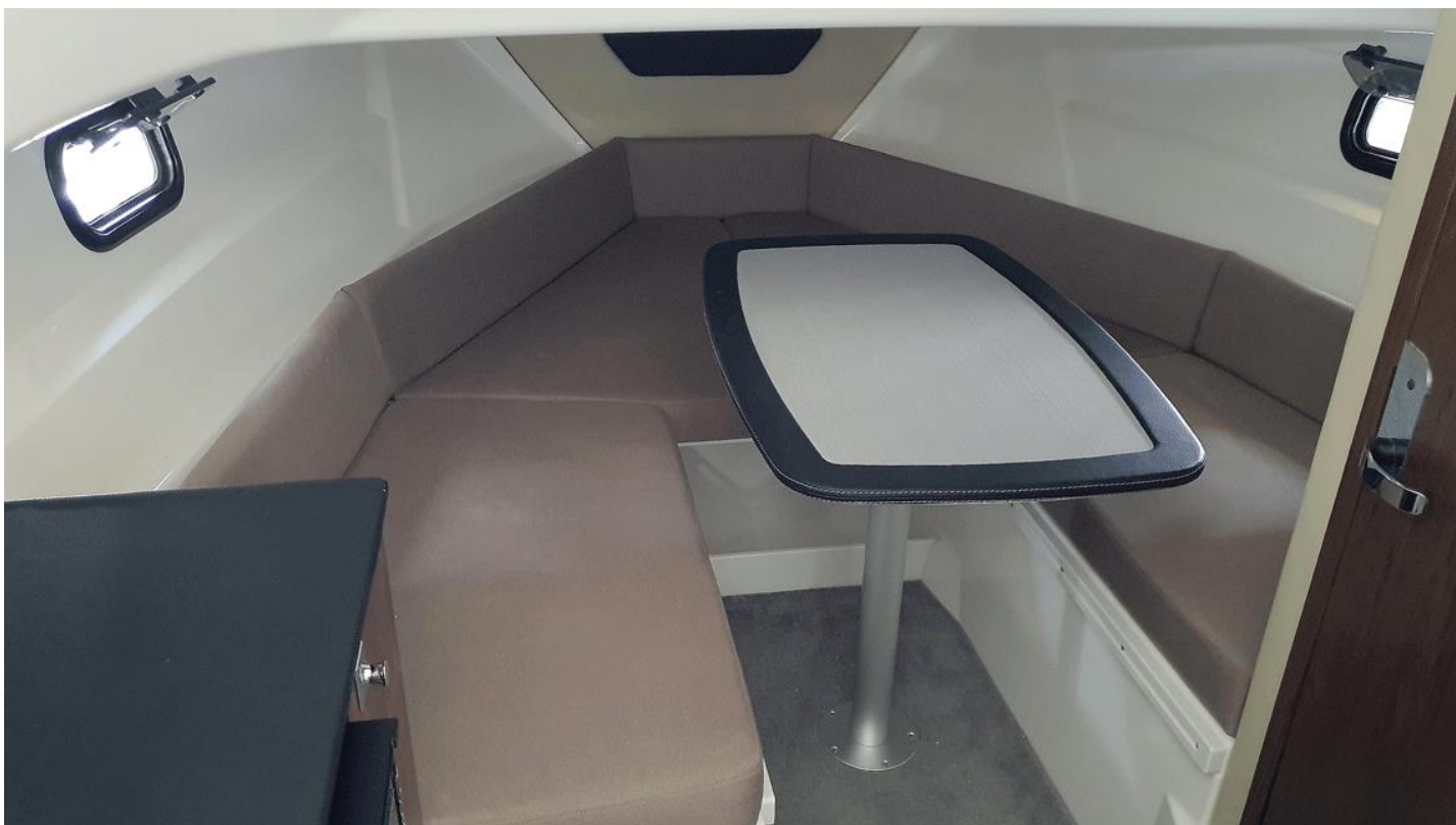
The Interior is enlarged, Bigger rectangular Port Holes. The walls and ceilings are fiberglass Gelcoat finish instead of the old carpet finish.
